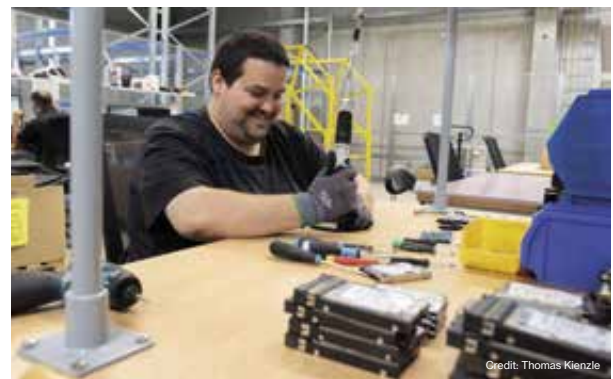
AfB employee Manuel Garcia takes apart a hard drive.
